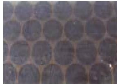
M01: Dark brown discoloration of EVA encapsulant
