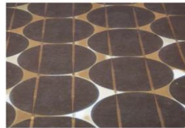
M07: Yellowing of encapsulant
